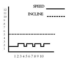
The **Cardio Program** is designed to vary the treadmill Speed, while maintaining a constant Elevation.
